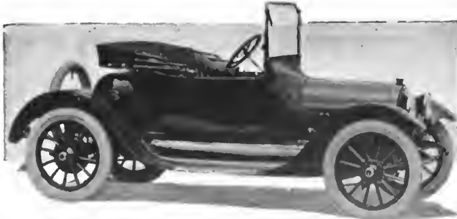
Small four-cylinder roadster Buick model C-24, selling at $900. Note the new rain-vision ventilating windshield
